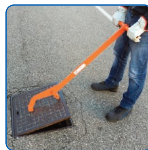
● Lifting - Pulling The long dimension of the lever limits the lifting effort
